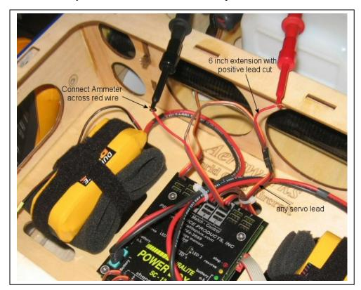
You need to have the ability electronically adjust the centers and endpoints of each servo to properly match them and this Model SC-2 Powerbox has this programming capability built in. Obviously, each radio manufacturer sells devices that also facilitate this so use whatever works with your equipment or suits your needs.
