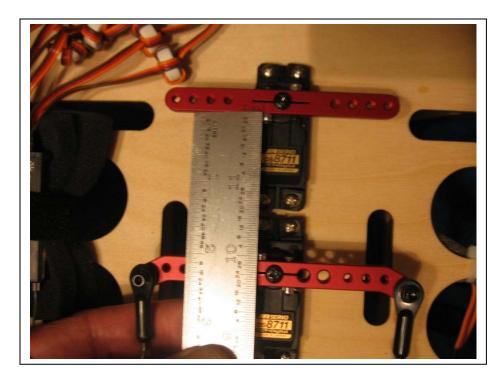
Once you have accomplished this, it's time to attach some linkage between the two servos so that you can double the torque to the rudder. I measure between the appropriate forward and aft servo arm holes (make sure they are at the exact same radius!) to determine the proper linkage length. Then I fabricate the linkage and attach it to the aft servo arm on one side. I temporarily affix it to the forward servo arm and observe any
